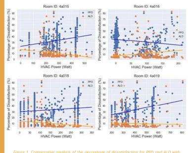
Figure 1. Comparative analysis of the percentage of dissatisfaction for PPD and ALD with respect to HVAC power use per zone of the living lab. The blue and orange lines show the linear regression of the data points for the PPD and ALD, respectively.
