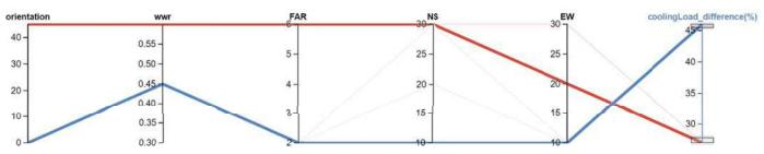
Models with minimum and maximum percentage difference in cooling load
